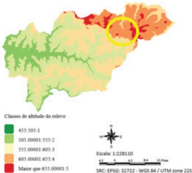
**Figure 2.** Hypsometric map using the soil elevation model of the municipality of Taquaritinga, SP.
