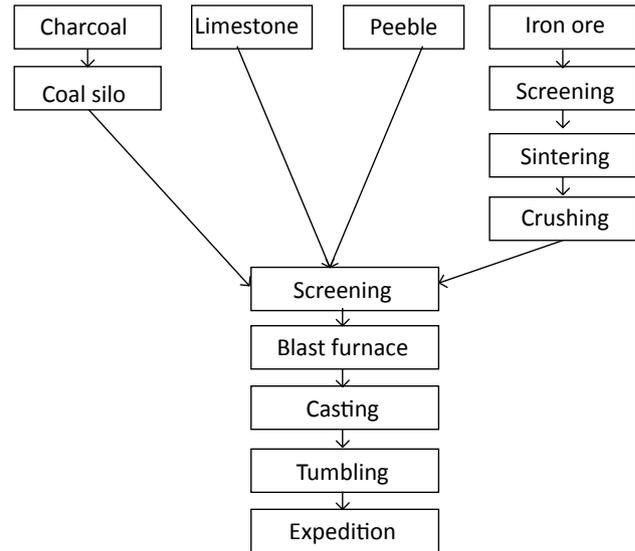
**Figure 1** - Summary of the pig iron production process - Marabá Steel Factory.
