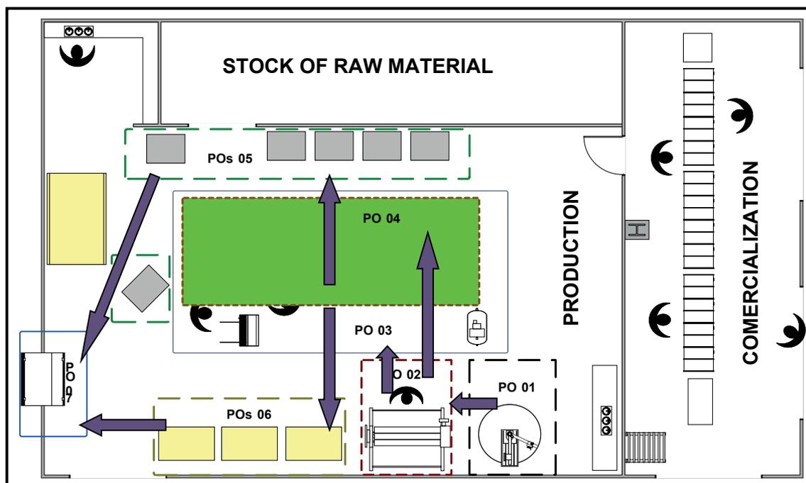
Figure 2. Approximate Disposition of Operational Stations in Bakery Layout
